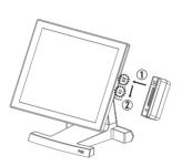
Please close I/O cover after inserting the cable into COM6/USB port of I/O ports.
